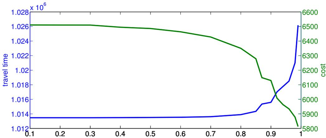
**Figure 2:** Cost vs travel time in Potsdam. Varying the weight parameter  $\lambda$  ( $x$ -axis) results in line plans with different costs (green) and travel times (blue). A value of  $\lambda = 0.1$  almost ignores costs, a value of  $\lambda = 1$  ignores travel time.
