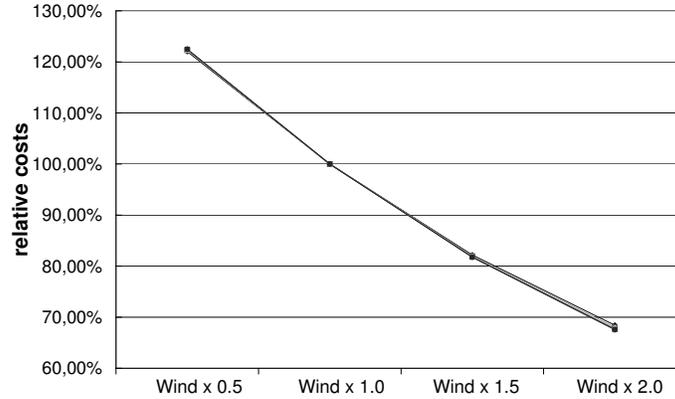
**Fig. 1.7.** Minimal expected costs depending on the wind power capacity installed for different storage capacities installed.
